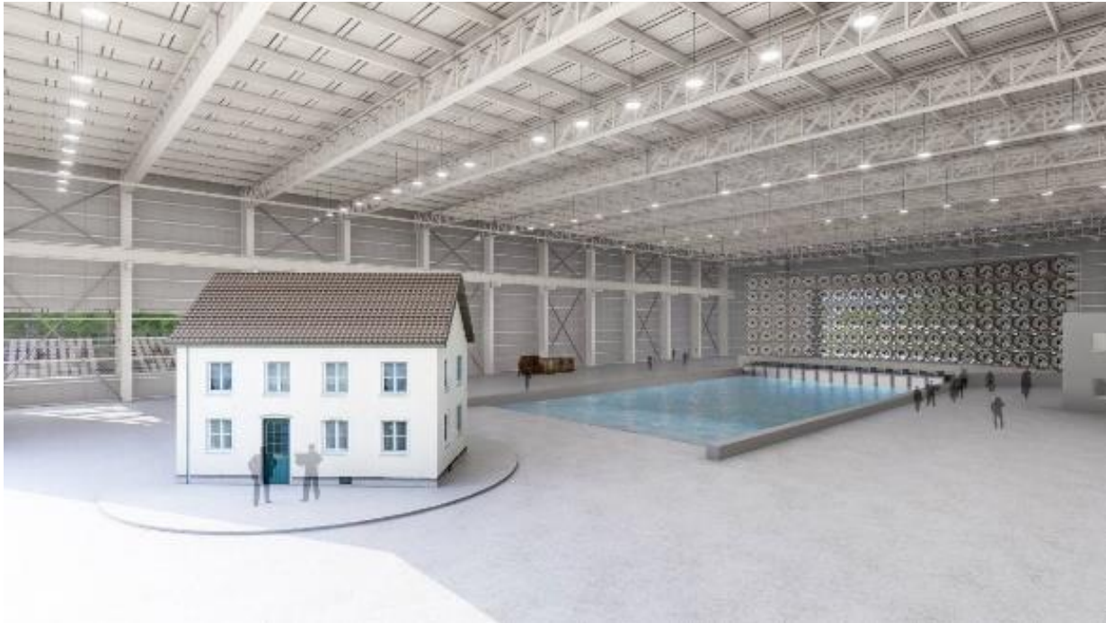
Figure 2. Visualization of the interior of the “Full-Scale 200 mph Wind and Wind-Water Testing Facility.”
