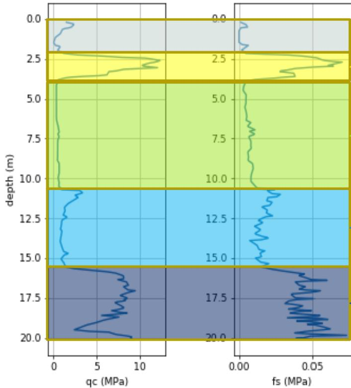
Small layer thickness, boundary effects at top and bottom
